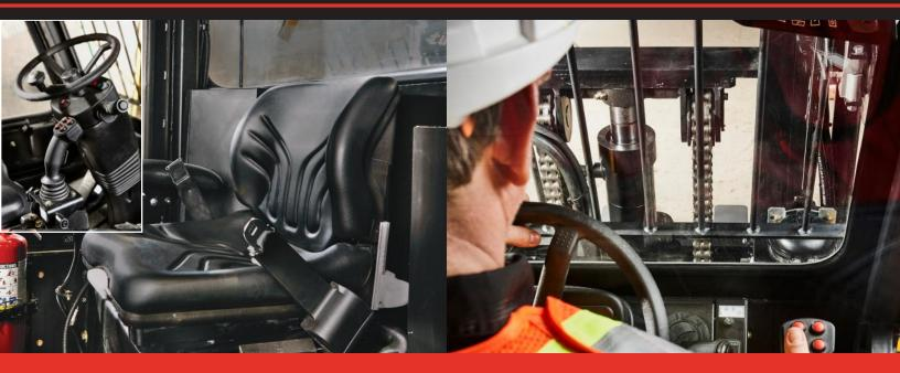
The cab interior houses ergonomic controls, like the multifunction joystick, and a colour display monitor that enable the operator to maneuver comfortably and safely. The full-view cab is devoid of channels in rear corners to eliminate blind spots and increase all-around and upward visibility.
