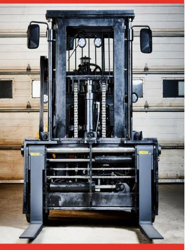
The heavy-duty, high-visibility mast allows for safer operations as it provides an optimal view of the loads and forks, and the mining worksite altogether.
