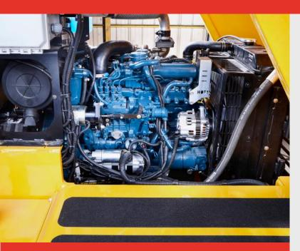
The engine hood opens mechanically and can be completely removed for ease of service.
