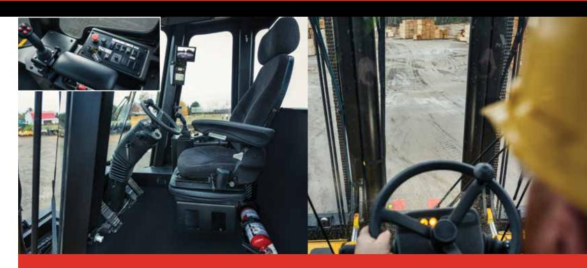
The cab interior is wide, long and tall to give the operator more space and a comfortable ride. It also includes ergonomic controls, a multifunction suspension seat and an optional colour display monitor. The full-view cab is equipped with an overhead window and is devoid of channels in rear corners to eliminate blind spots and increase all-around and upward visibility.
