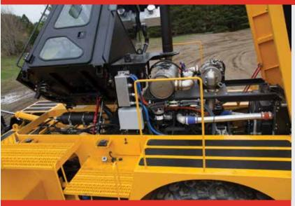
The engine hood opens mechanically, and can be tilted, along with the cab, for ease of service.\*
