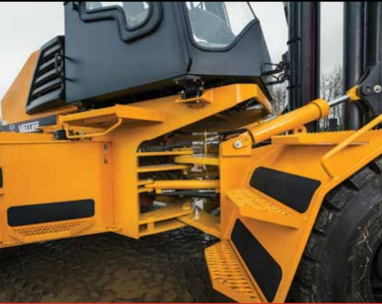
These lift trucks boldly go where no standard lift trucks can. Their compact size and articulated features make them ideal for squeezing into tight and confined spaces. E.g. a 4DA20C handling a pallet of timber 12 feet wide by 4 feet long can operate in narrow 19-foot aisles.
