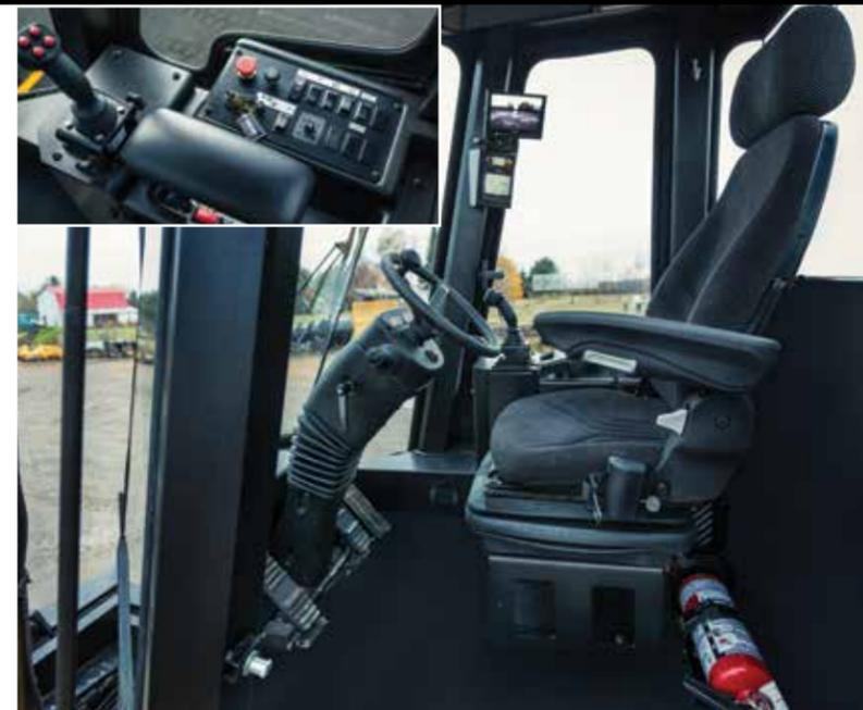
The cab interior is wide, long and tall to give the operator more space and a comfortable ride. It also includes ergonomic controls, a multifunction suspension seat and an optional colour display monitor.
