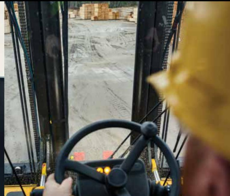
The full-view cab is equipped with an overhead window and is devoid of channels in rear corners to eliminate blind spots and increase all-around and upward visibility.
